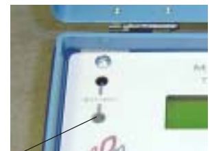
Battery Charge Indicator
