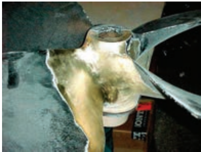
Removes heavy barnacle buildup and 2-part epoxy base coat.
