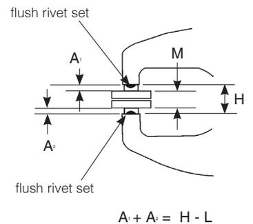
If necessary, select rivet sets a little short and shim to the correct length using spacer shims.
